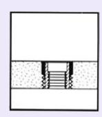
Same size replacement insert may be installed in the original hole.
