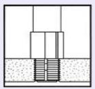
Drive keys down with several hammer taps on the proper installation tool
