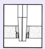
Remove inert using Helisolid drill out tool
