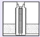
Tap new threads with a standard tap. See charts for proper size and depth.
