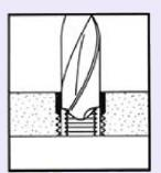
Drill out material between keys and internal thread with standard drill to specified depth (refer to charts for proper dimensions)
